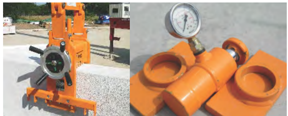
Fig. 5: WKV Lifting Clamp and Manometer.
